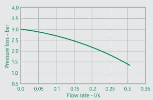
Reference conditions: upstream pressure = 8 bar downstream pressure = 3 bar
